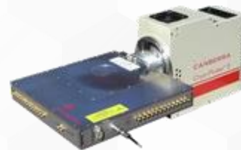
Planar DSSD HPGe detector electrically cooled for gamma-ray imaging
