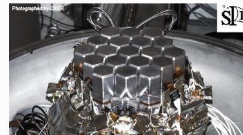
INTEGRAL/SPI - array of 19 encapsulated HPGe
