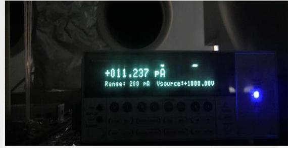
Immerse the detector into liquid nitrogen for about 8 hours, we got a stable leakage current  $\sim 10$  pA for 1000V bias voltage.
